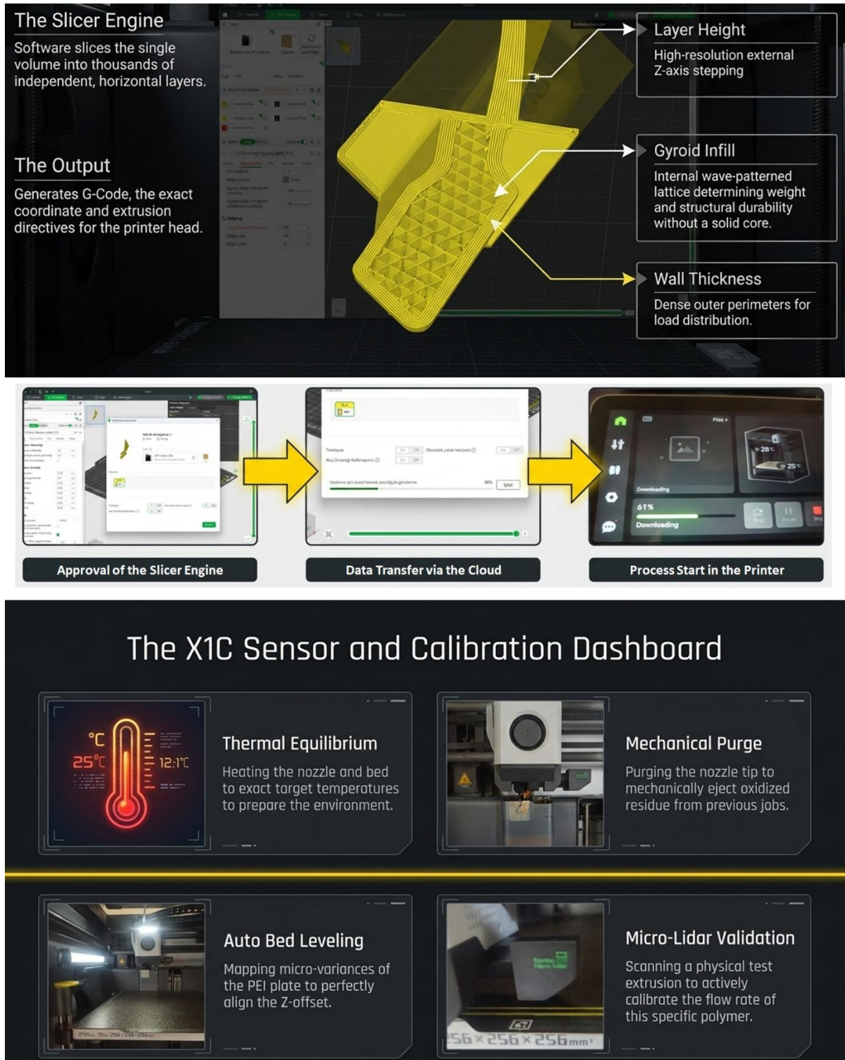
Figure 4.6 Main steps in the model slicing and process preparation stages.
